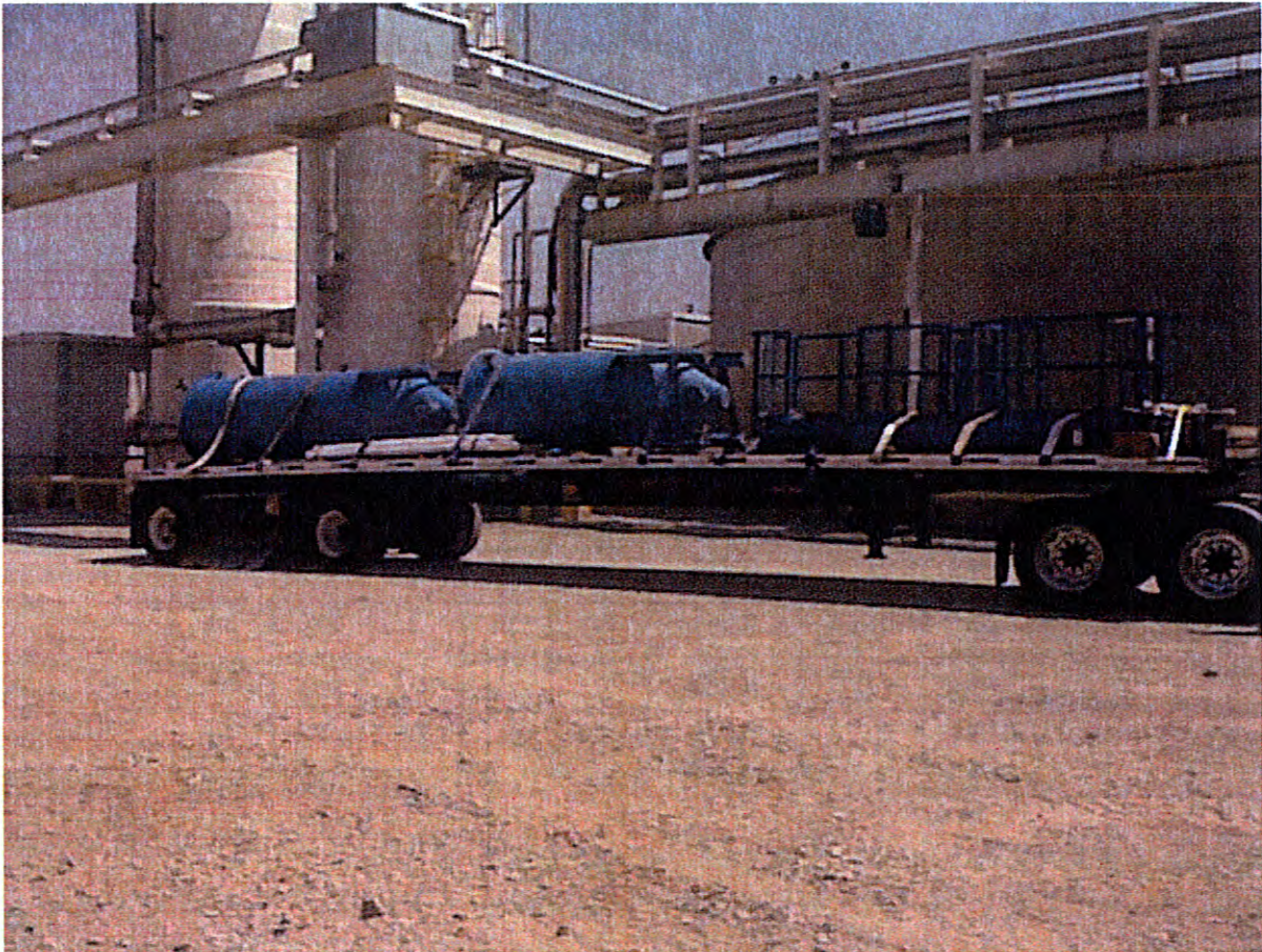
Figure 8 Parkson D2 Sand Filters (Foreground on trailer)
